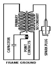
the same point, the reversal of magnetic polarity, in turn reverses the induced current. So a rapidly rotating magnet pair causes a rapid collapse of the core's magnetic field, this in turn induces a large voltage spike in the primary winding, which may be as high as 200 or 300 volts.
